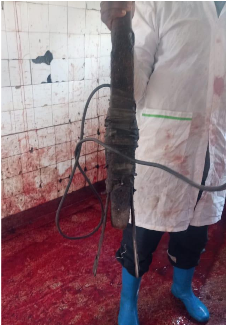
Figure 6; An image showing the electrode set that was used for stunning.
