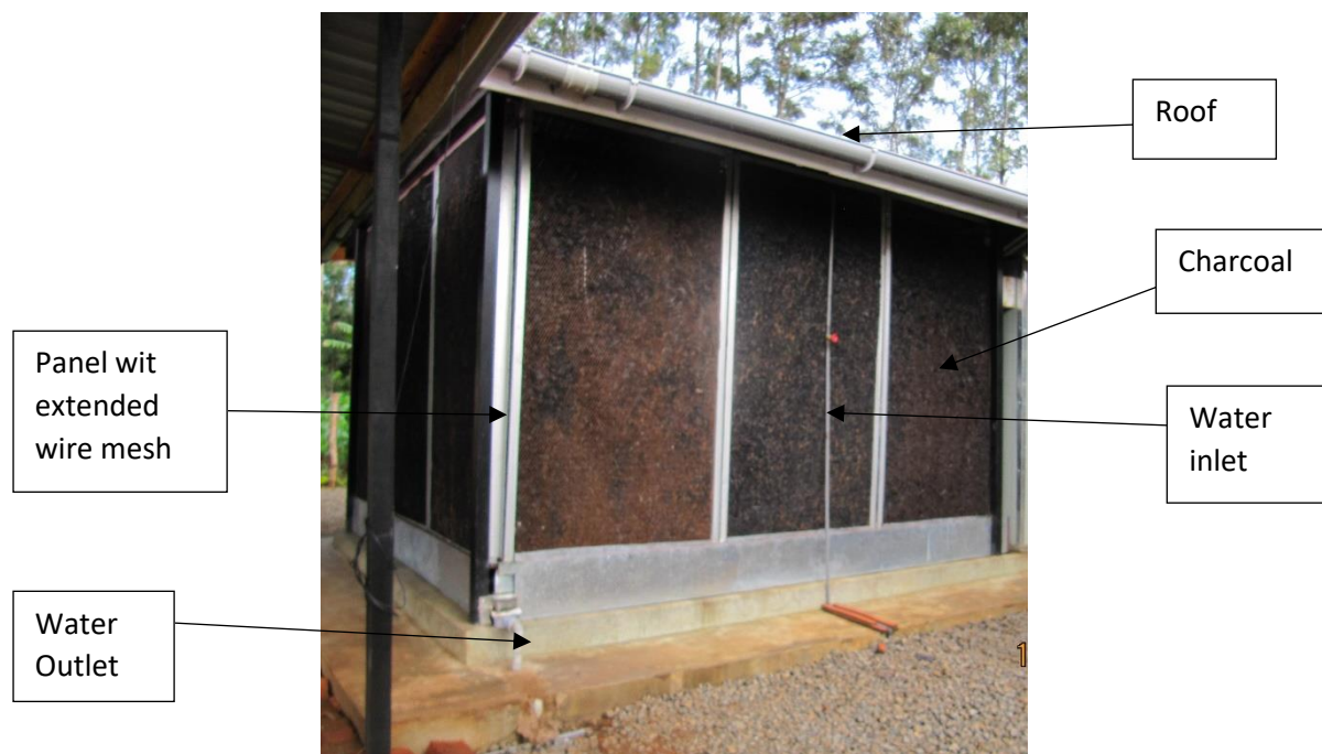
Figure 2.5: Evaporative Charcoal cooler (Source: Karurumo Smallholder aggregation and processing center, Embu County).
