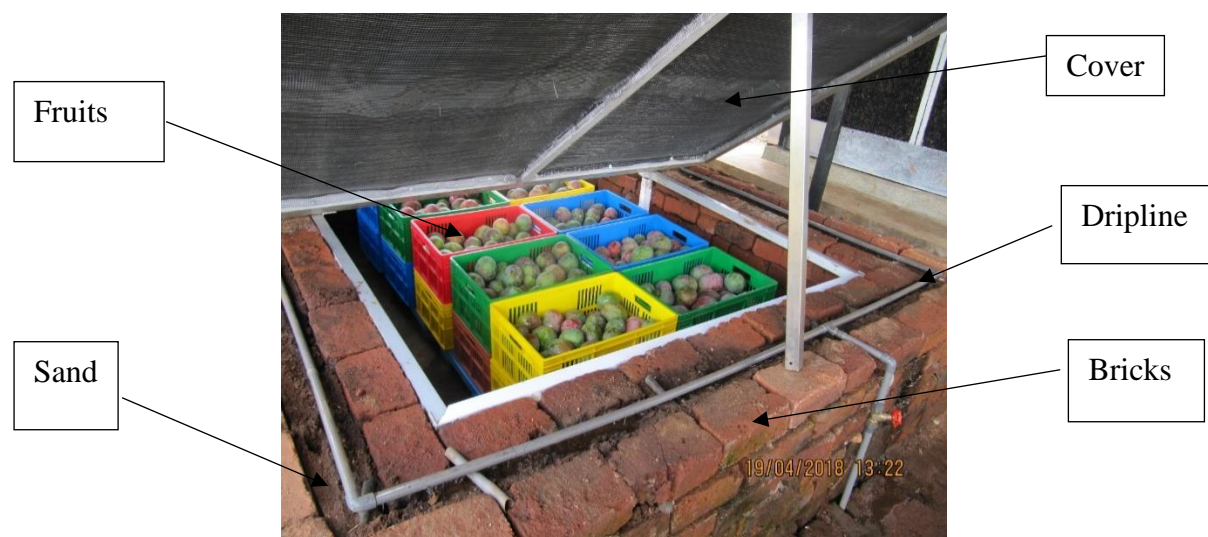
Figure 2.4: The Zero Energy Brick Cooler (Source: Karurumo Smallholder aggregation and processing center, Embu County)
