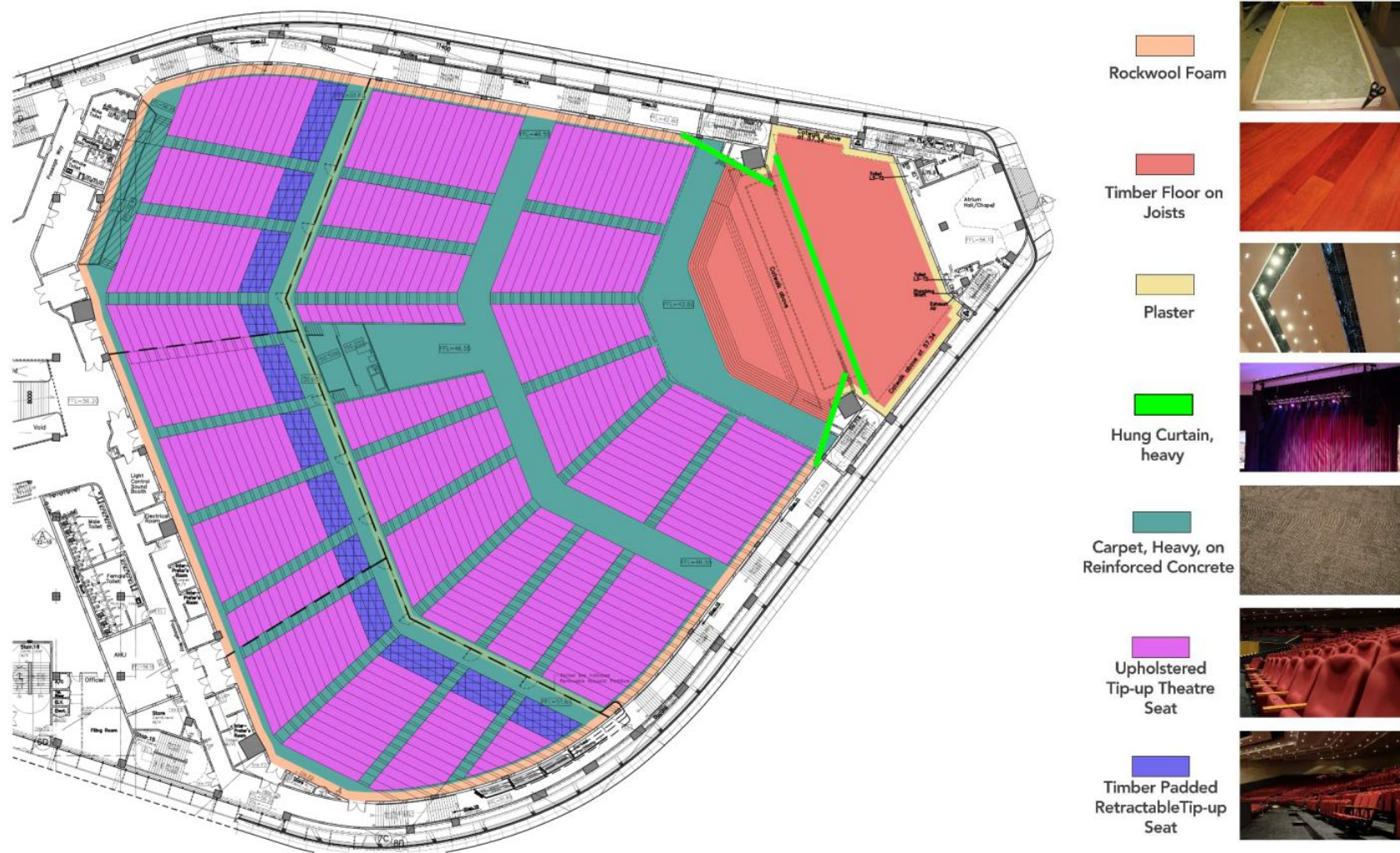
Figure 48. Calvary Church: Wall & ceiling surface finishes in plan.
