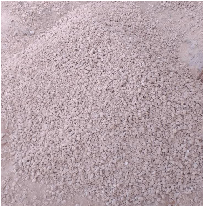
Figure D.9: Crushed Course Aggregate From Limestone Rock
