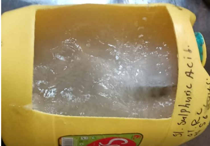
Figure 3.8: Samples Exposure 5 % Sulfuric Acid solution (H 2 SO 4 )
