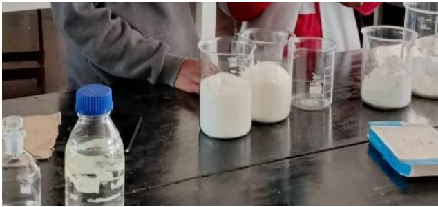
Figure 3.7: Magnesium Sulphate Powder (Left) and Samples Exposure 5% Magnesium Sulphate Solution (Right).
