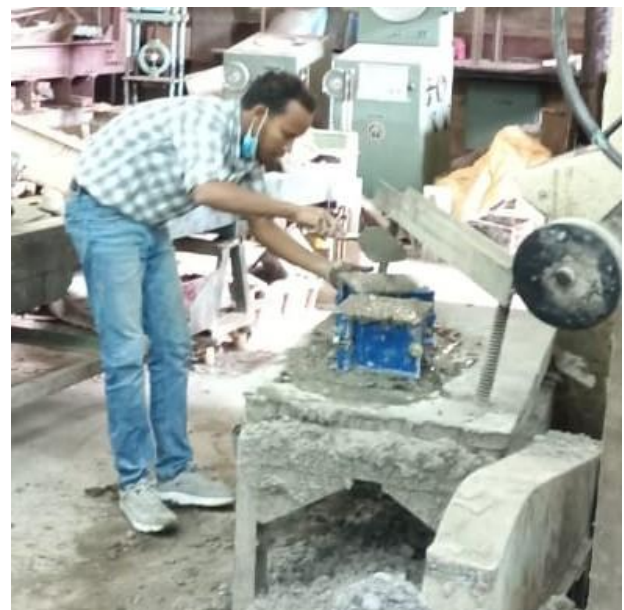
Figure 3.5: Compacting of Concrete Cubes for Strength Tests
