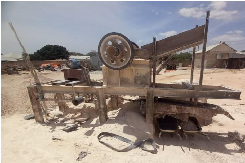
Figure D. 7: Material Used for Crushing the Limestone Rock
