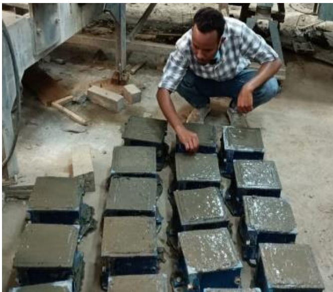
Figure 3.4: Preparation of Concrete Specimens
