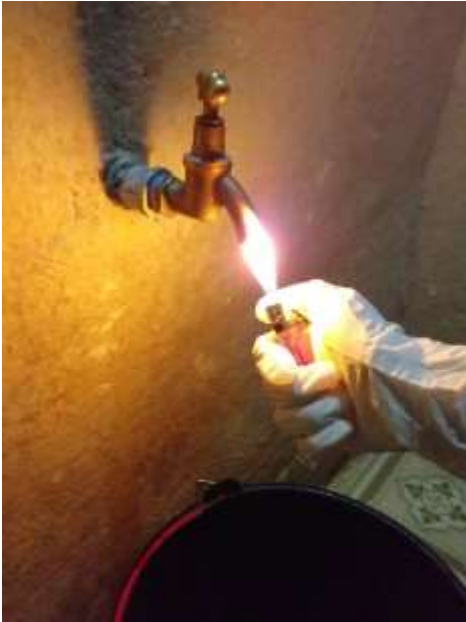
Figure 2 Sterilizing pipe before collecting water samples
