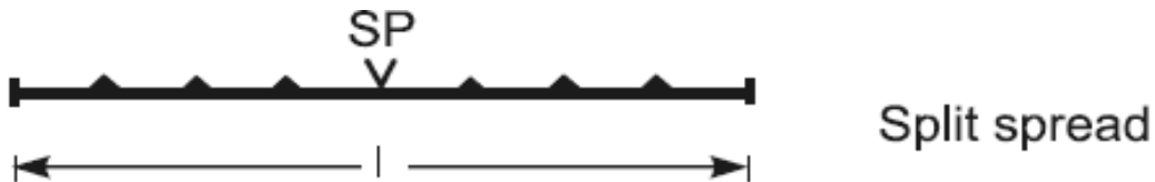
Figure 3.3: Commonly used source-geophone arrangements (spreads) for 2D seismic reflection data acquisition (Schuck and Lange, 2007).
