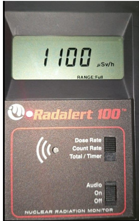
Image 6: Survey meter showing high reading at control lead glass
