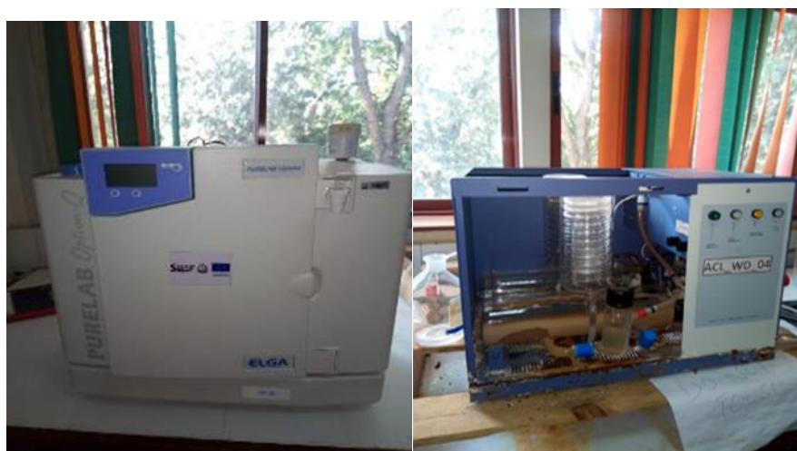
Figure 3. 2: A picture of ELGA water de-ionizer (left) and Aquatron double distiller (right)
