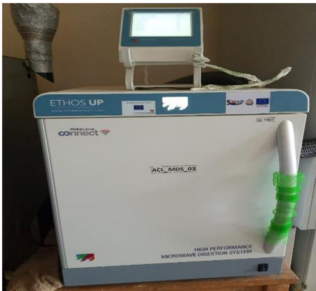
Figure 3. 3: A photograph of ETHOS UP® high-performance microwave
