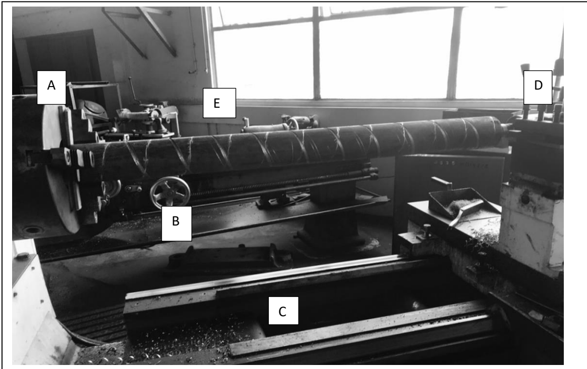
Figure 3.3: Machining the model chimney to create 4inch pitch of 10mm thickness where copper tube was fitted.
