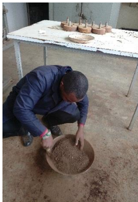
Plate 3-7: Mixing FCD with soil
