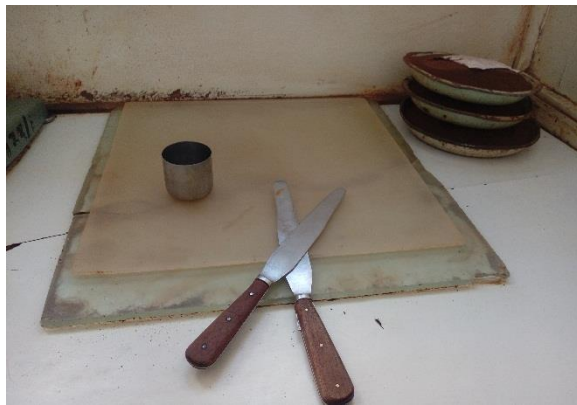
Plate 3-20: Atterberg Limits apparatus
