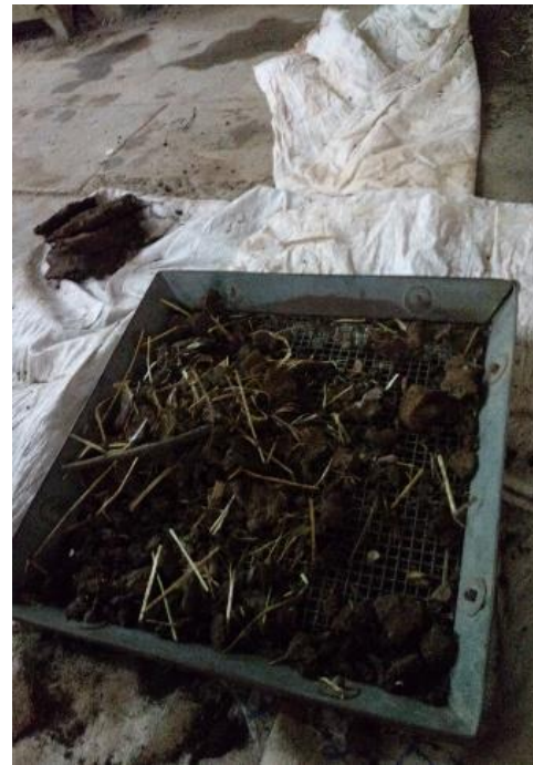
Plate 3-2: Sieving using a 20mm sieve
