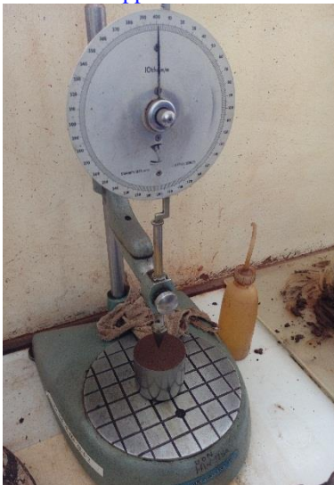
Plate 3-24: Testing for Liquid Limit
