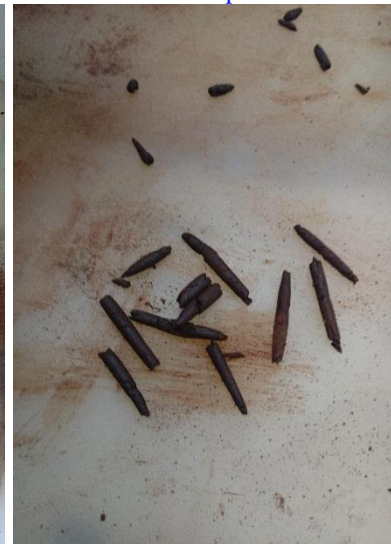
Plate 3-26: Sample for plastic limit
