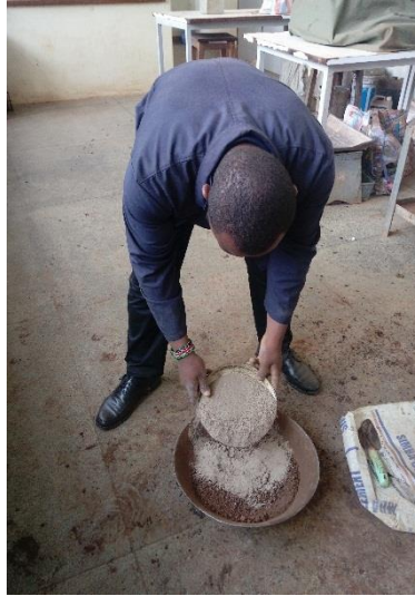
Plate 3-14: Mixing CDA with soil
