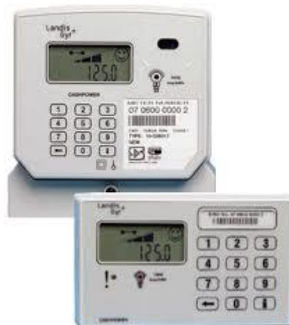
Figure 1.2: Customer Interface Unit [3]
