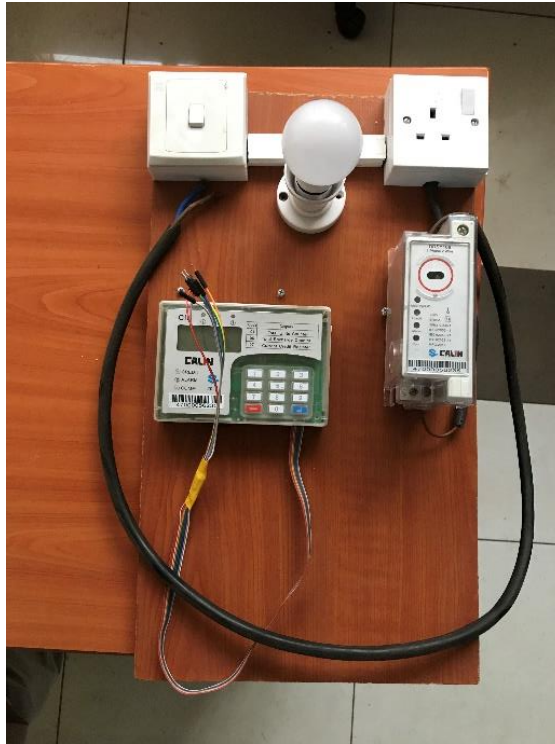
Figure 4.1: Sample meter board
