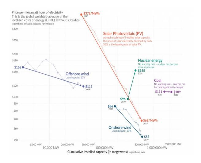
Figure 1. 2: Weighted-average (LCoE) with increased installed capacity (IRENA, 2020)
