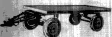
5-TON TRAILER This robustly built All-steel Trailer is constructed to a body size of 14 ft. x 7 ft.
