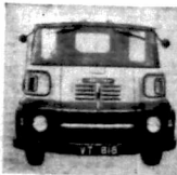
Increased visibility! Large windows at front and rear enclose "blind spots" to a minimum.
