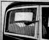
This view shows two items of interest: (P) The flush-type direction indicators with automatic return; (R) The new-type rear window hinged from the body pillar, giving ventilation without draught.
