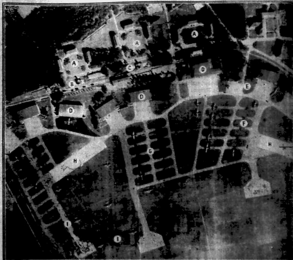
Another R.A.F. photograph of the Langen Haagen Aerodrome, ten miles north of Hanover. The key to the annotation: A. Quarters; B. Special Railway line for aerodrome; C. Station and platform; D. Hangars; E. Motor transport; F. Oil patches made by aircraft parked at the same spot always; G. Servicing tarmac; H. Runway; I. Aircraft just moved off across aerodrome.
