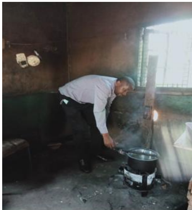
Figure 3.4: Water Boiling Test Set Up
