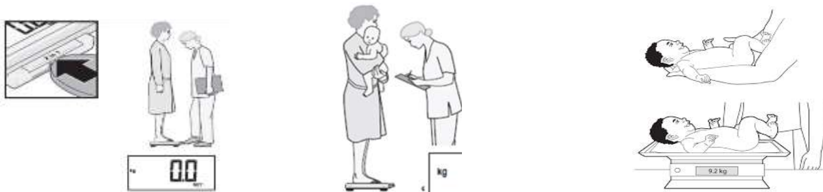
Figure 4: Weight measurement using electronic mother/child and infant scales
