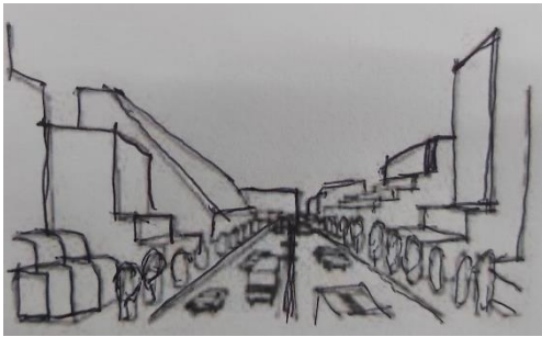
Figure 241 Image showing street canyons with stepped buildings to the back of the streets.
