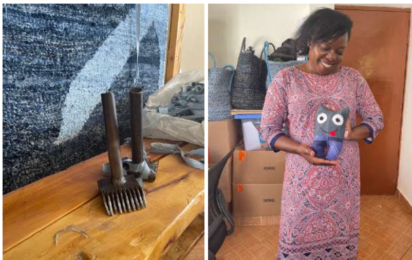
Figure 14: SME2 (left) Weaving comb tools made of iron against a rug made of 100% recycled second-hand jeans.
