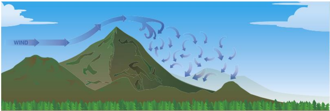
Figure 5: Schematic illustration of turbulence in mountainous regions (Aviation Handbook, FAA)
