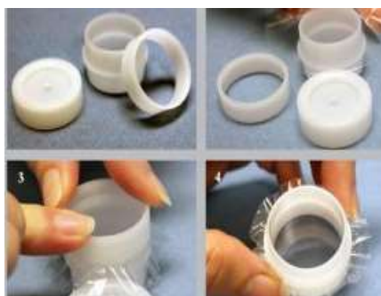
Figure 3.4: Preparation of XRF sample cups
