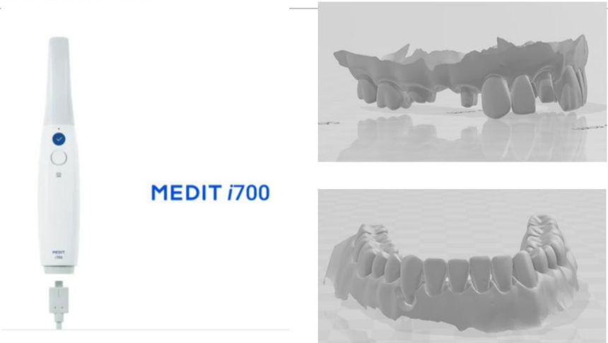
Figure 4.4: Sample measurements done using impressions from Medit i700 digital scanner
