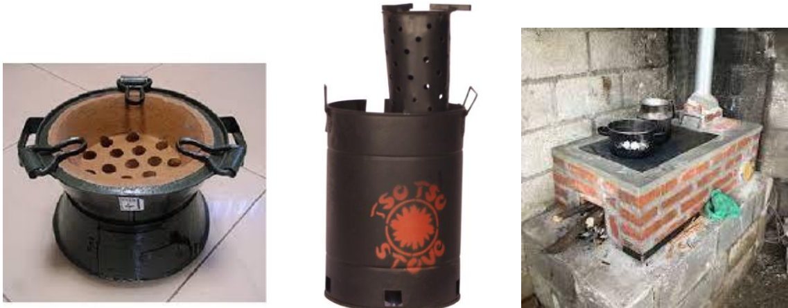
Plate 1: The ceramic jiko (left) and the Tsotso jiko (middle) and Justa stove (right) Source: Global Alliance for clean cookstoves, new dawn engineering & stoves online
