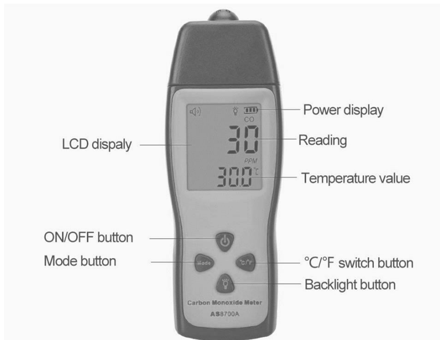
2 Figure 3.3. Diagram illustrating the various parts of the Carbon Monoxide Meter
