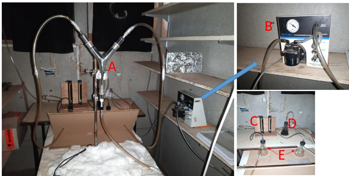
Figure 16: An olfactometer choice experiment setup. Y-tube olfactometer (A), electric Air Cadet Vacuum/Pressure Station (B), Flow Rate regulators (C), air charcoal filter (D), sample chambers (E).
