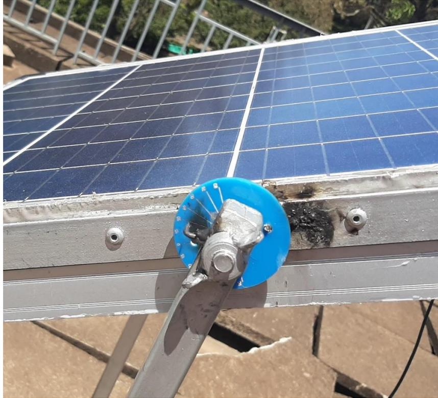
*Figure 4.2: The calibrated angle scale fitted to the module's frame.*
