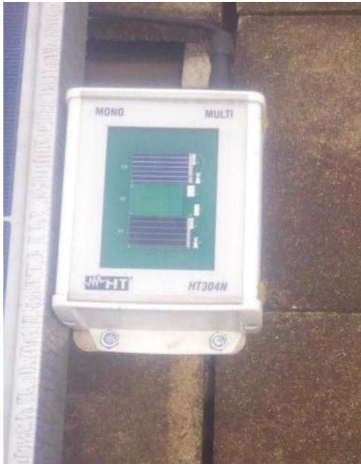
*Figure 4.3: The HT304N Reference Cell is mounted to the module frame.*
