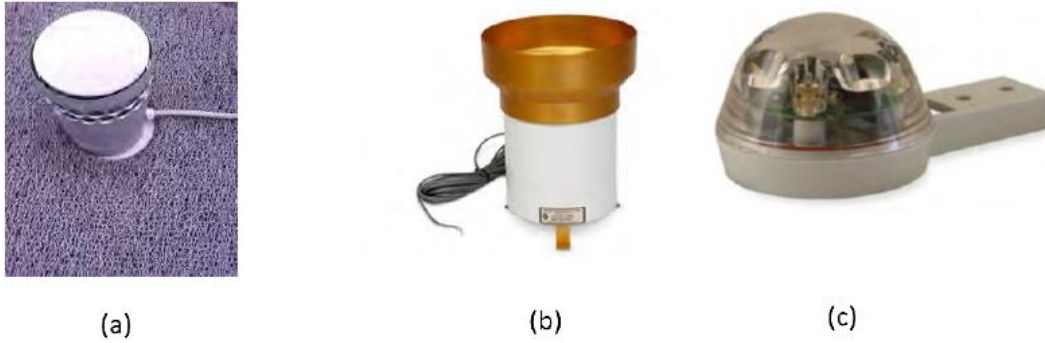
Figure 3.3: Instruments for measuring rainfall include (a) disdrometer, (b) tipping bucket rain gauge, and (c) an optical rain gauge [63] [64]
