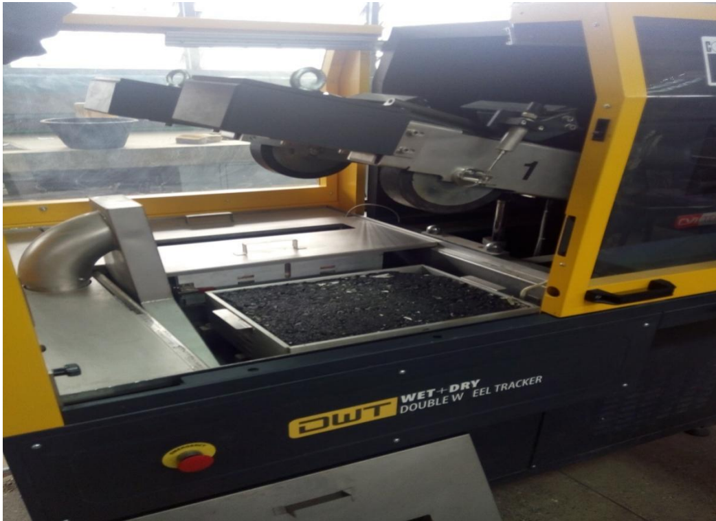
Figure 3.10: Performance testing using wheel track tester
