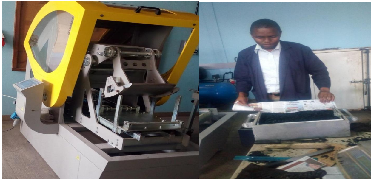
Figure 3.9: Preparing samples for roller compaction in the laboratory
