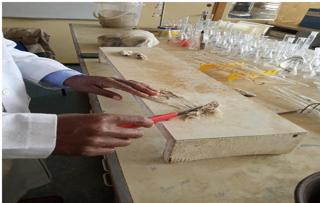
Plate 4-4: Assessment of the unhairing and appearance of the pelt by scrapping the epidermis
