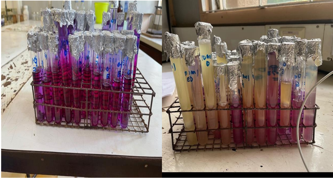
Figure 4.16b: MPN analysis of water samples of Ndakaini dam in wet season, before and after incubation
