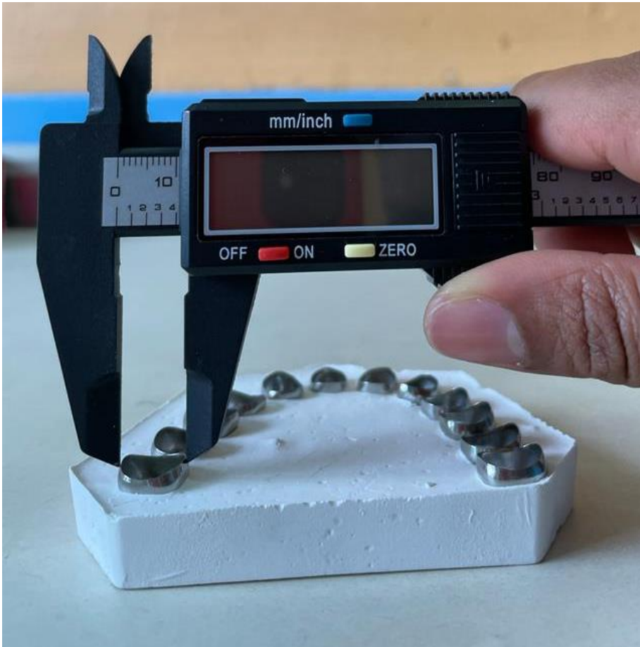
Figure 9 (Appendix IV b); Showing mounted SSCs of different sizes for the same tooth, and the measurement of the BL dimensions of the Stainless steel crowns
