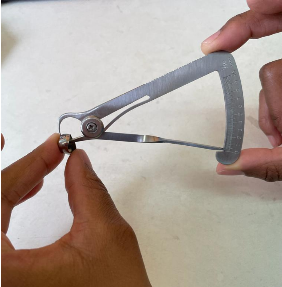
Figure 10 (Appendix IVc); Measuring the thickness of the stainless steel crowns
