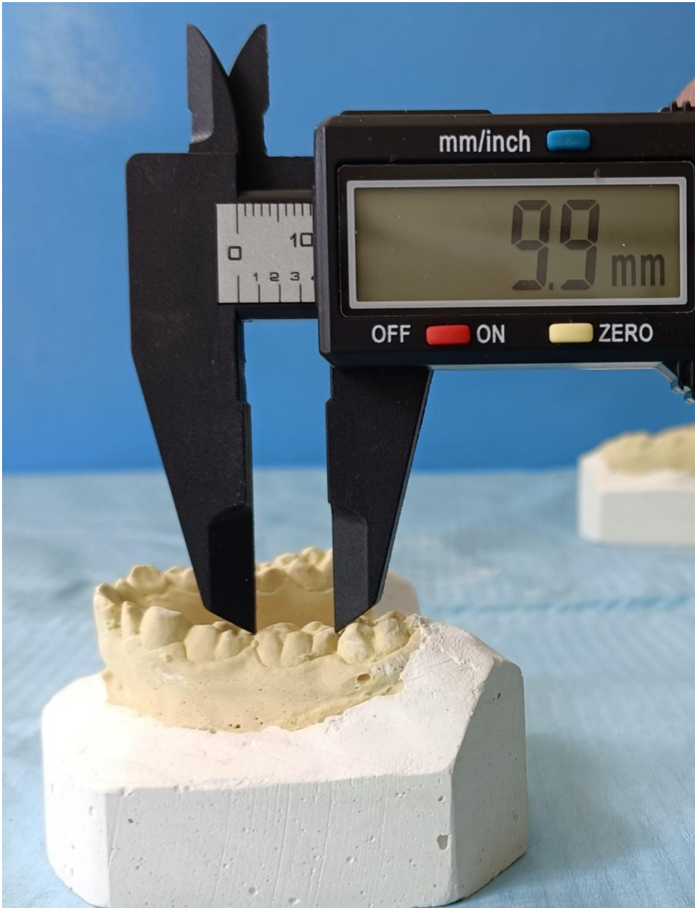
Figure 6 (Appendix IIIa) Measurement of the mesiodistal tooth width
