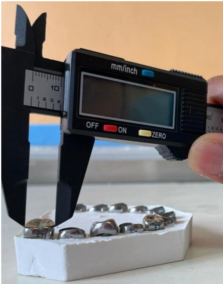
Figure 8(Appendix Iva); An example of one of the models, showing the mounted SSCs of different sizes for one tooth and the measurement of the MD dimension of the Stainless Steel crowns
