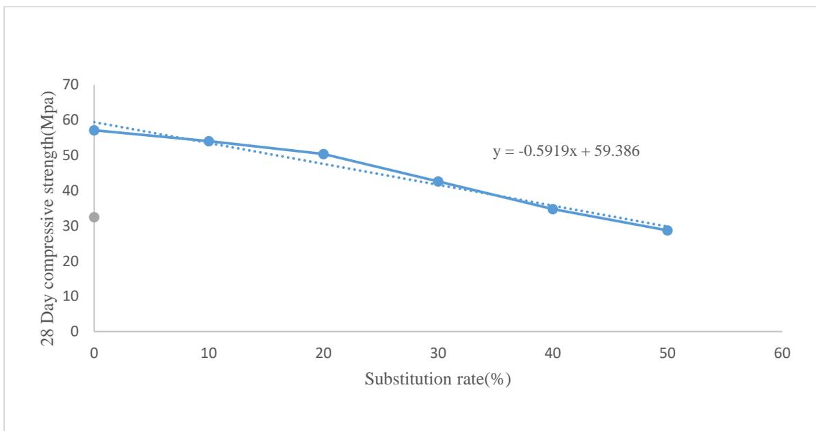
**Figure 7:** A graph of 28-day compressive strength against substitution rate.
