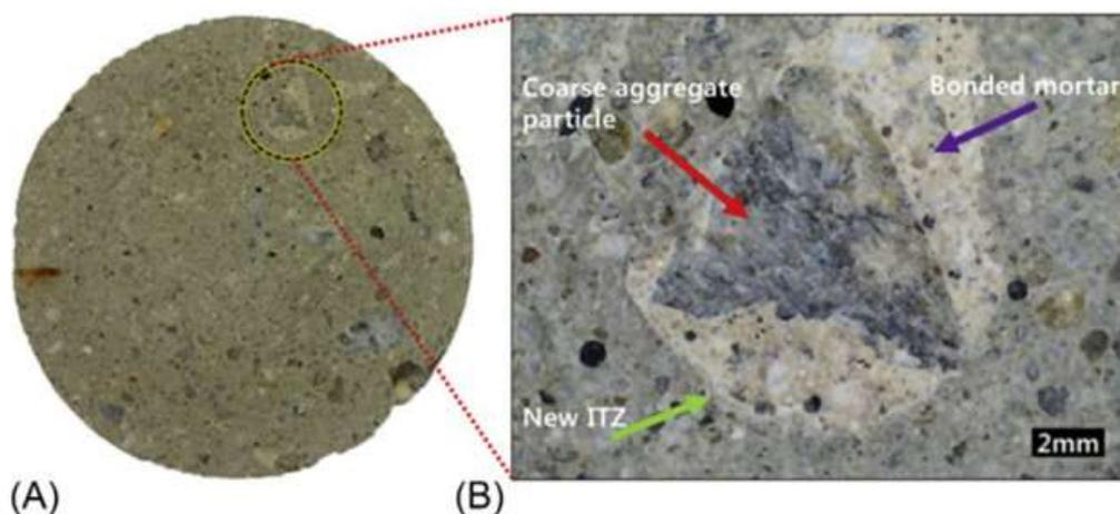
**Figure 1:** (A) Mortar adhered on coarse aggregate, (B) magnification of adhered mortar on coarse aggregate showing bonded mortar, coarse aggregate particle, and interfacial transition zones (ITZ)
