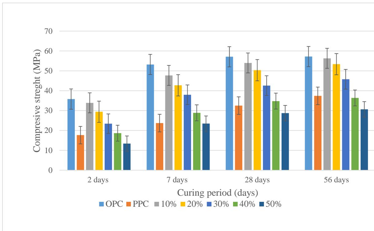
**Figure 4:** A graph of compressive strength against curing period
