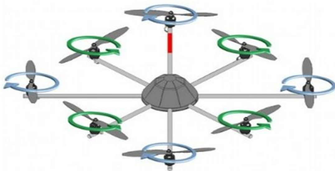
Figure 3.7 Propeller Installation and Direction of Rotation.
