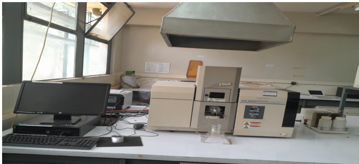
Fig 2.1: Schematic diagram of atomic absorption spectrophotometer
