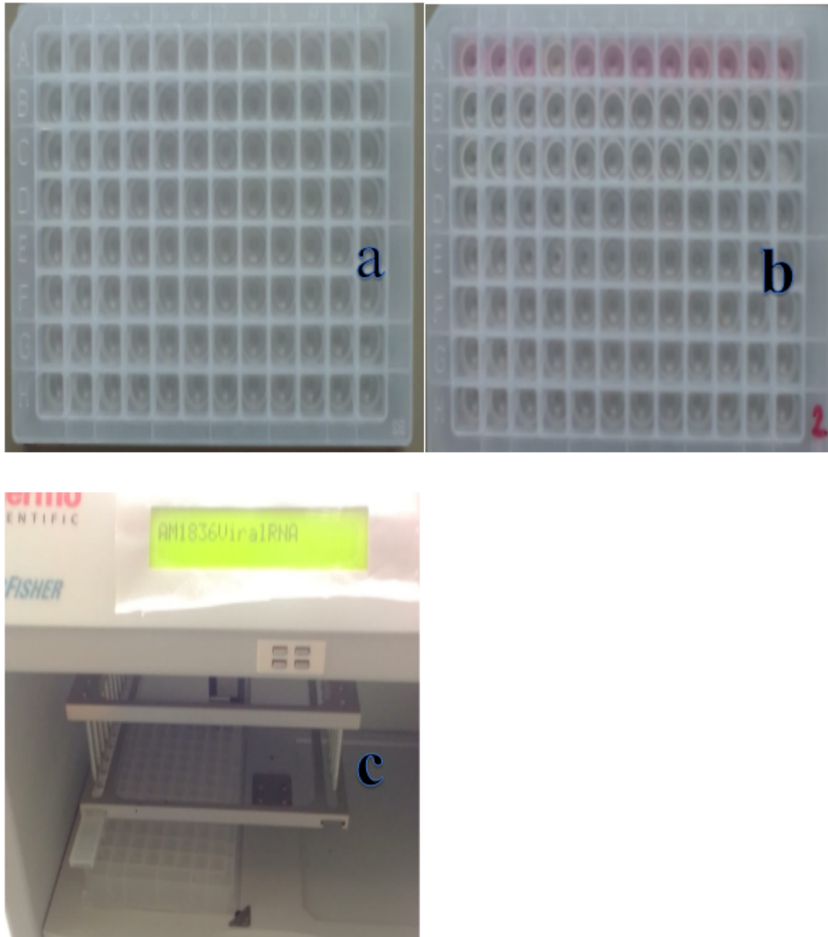
Figure3. 3: RNA extraction plates: (a) Empty plate with nine (A-H) rows having twelve wells each (1-12) (b) plate loaded with samples and reagents (c) plate inside MagMax total RNA extraction machine.
