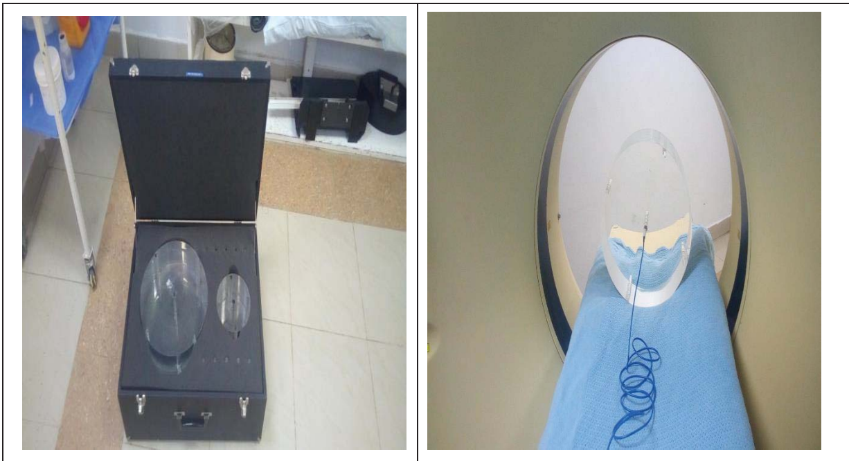
Figure 3.8: (A) PMMA (Body and Head) phantoms in the storage case, (B) PMMA Body Phantom connected with Pencil ionization chamber at the centre
