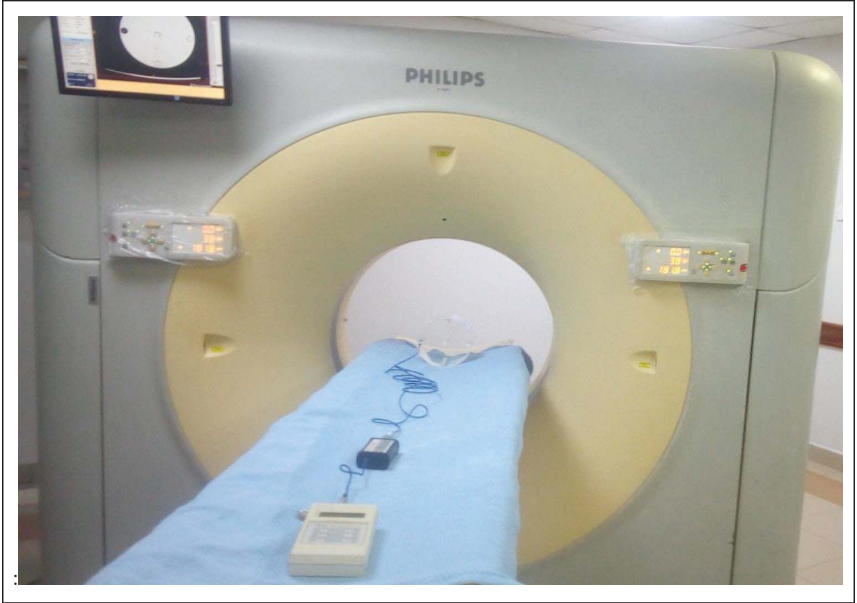
Figure 3.5: DIADOS E dosimeter (PTW, Freiburg, Germany) -to-PTW CT-adaptor-to-100mm pencil ionisation chamber for body phantom measurements
