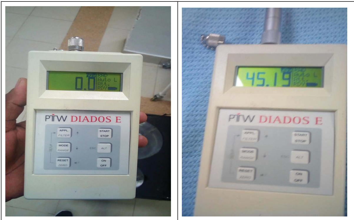
Figure 3.3: DIADOS E Dosimeter for Radiation Exposure measurements with Head Phantom
