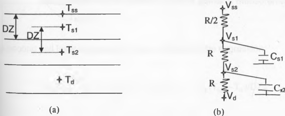
Figure 4.2: Heat flow and temperature regime in the soil layer (a). Left: Heat flow (b). Electrical network analogy
