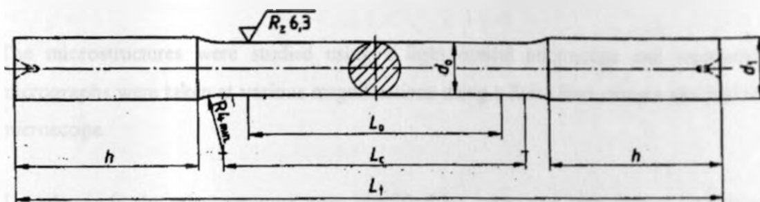
Fig 3.6 A DIN 50 125-A8X40 standard tensile test piece with a diameter d_0 of 8mm and an original gauge length L_0 of 40mm. Other dimensions are: d_1 - diameter of gripped ends (approx. 1.2 d_0 = 10\text{mm} ), L_c - parallel length ( L_0 + d_0 = 48\text{mm} ), h - length of gripped ends (30mm), and L_t - total length (115mm)
