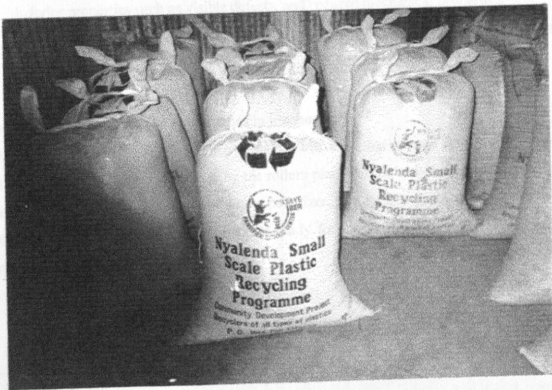
Plate 4.14: Shredded flakes packaged in 25-kg bags in NRP.
