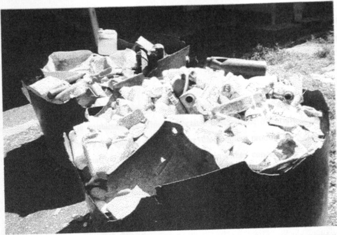
Plate 4.9: Grade sorted plastic wastes ready for shredding.
