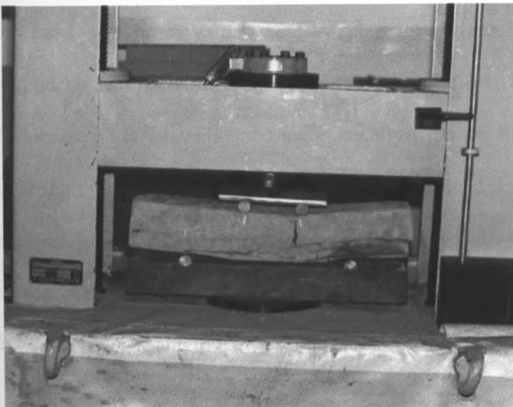
Plate 3.3 Flexural strength test of Sisal/RHAC composite beam in progress.
