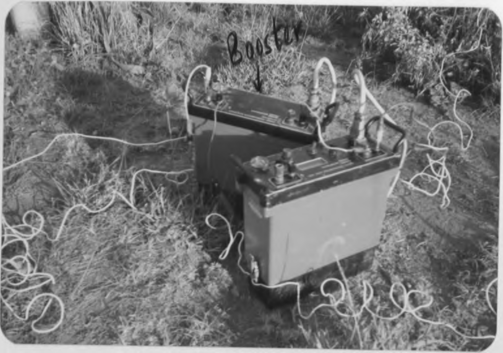
Plate 4 Close-up of the Terrameter with the Booster 'slaved' to the SAS 300 Terrameter.
