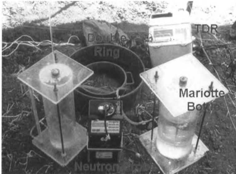
Figure 2.9: Double ring infiltrometer for measuring soil moisture regimes (Amoozegar and Warrick, 1986)
