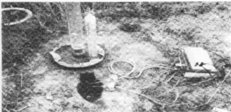
Figure 2.1: Disc infiltrometer fitted with minitensiometer (Vandervaere et al., 1997)
