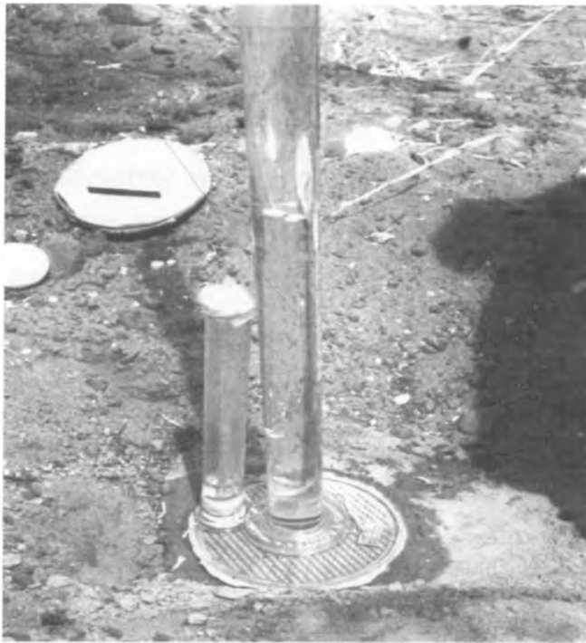
Figure 2.3: Disc permeameter (Perroux and White, 1988)
