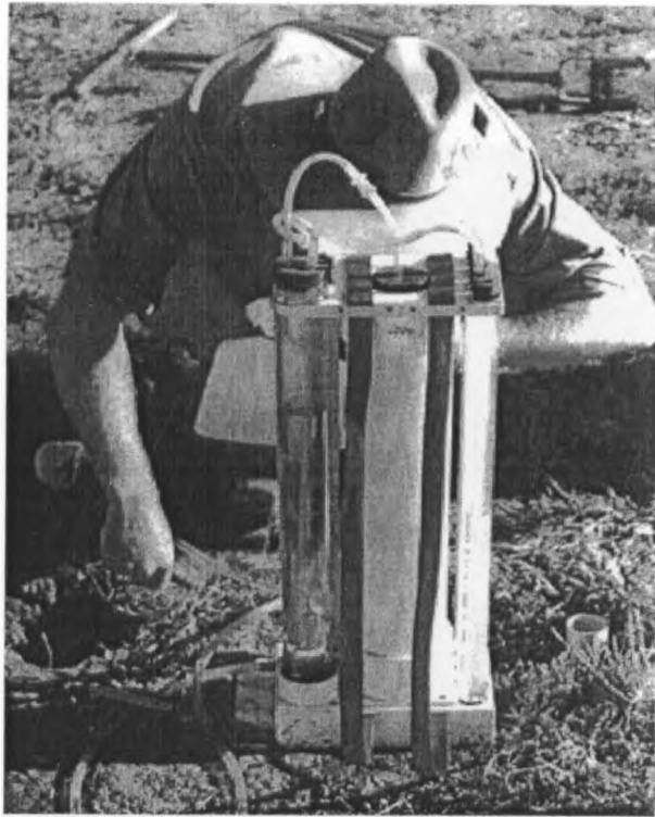
Figure 2.7: Borehole permeameter (Stephens, 1992)
