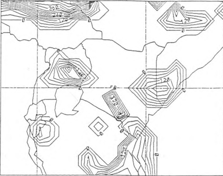
Figure 211: Convective precipitation rate at 1600 UTC (coarse grid). Contour values are in units of \text{m ms}^{-1} . Labels \times 1.0 \times 10^{-3} . Case with synoptic wind.
