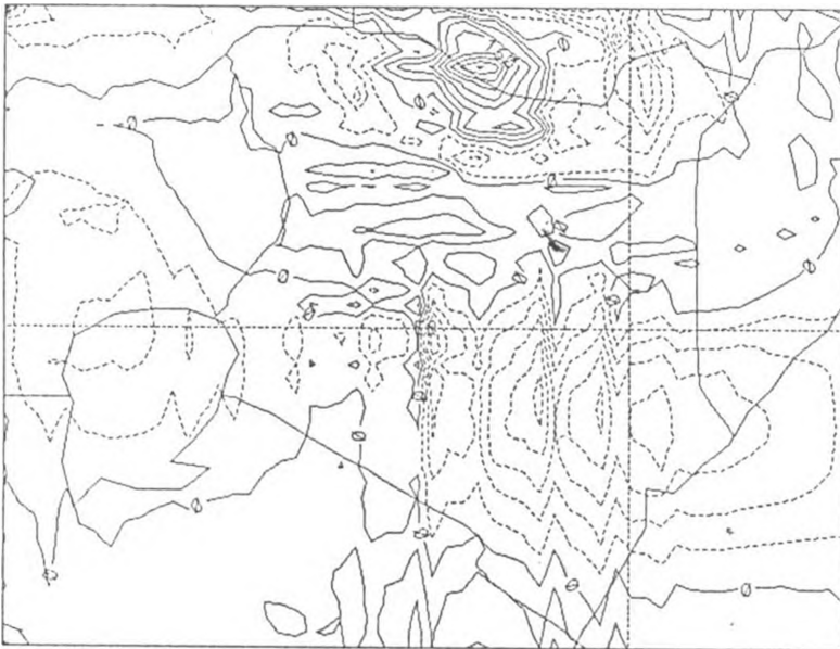
Figure 118: Vertical velocity field on terrain following coordinate 2.61 km above surface 1200 UTC (fine grid). Contour values are in units of \text{m s}^{-1} . Labels *1.0 \times 10^{-4} . Case with synoptic wind.
