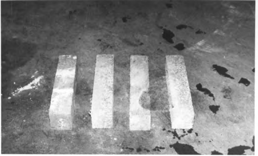
Plate 8.3 : Completely cured flexure beams ready for testing.
