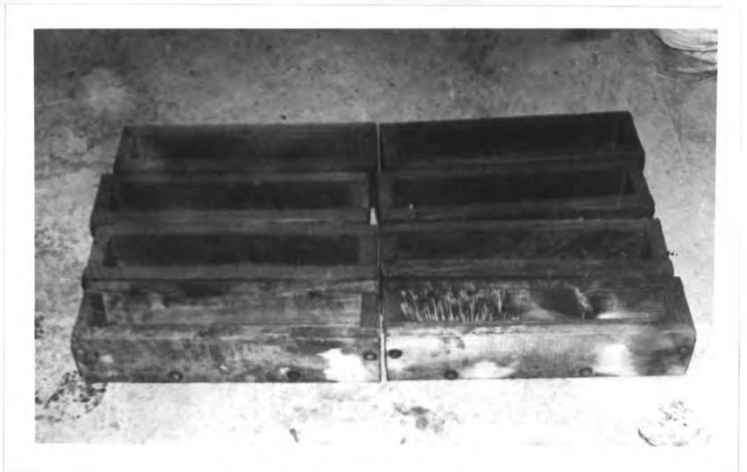
Plate 8.2 : Wooden moulds used for casting Tensile test samples
