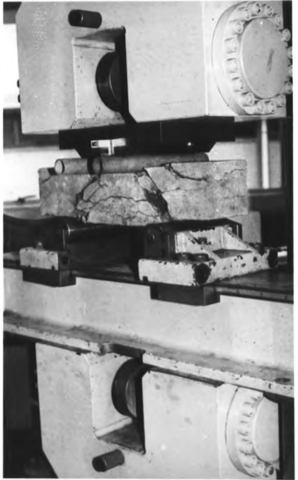
Plate 8.3 : Completely cured flexure beams ready for testing.
