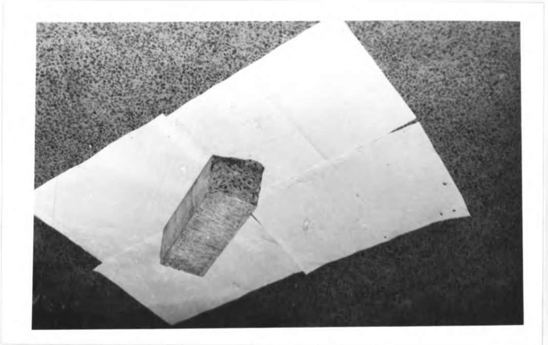
Plate 8.5 : Unreinforced samples after failure showing the failure surface
