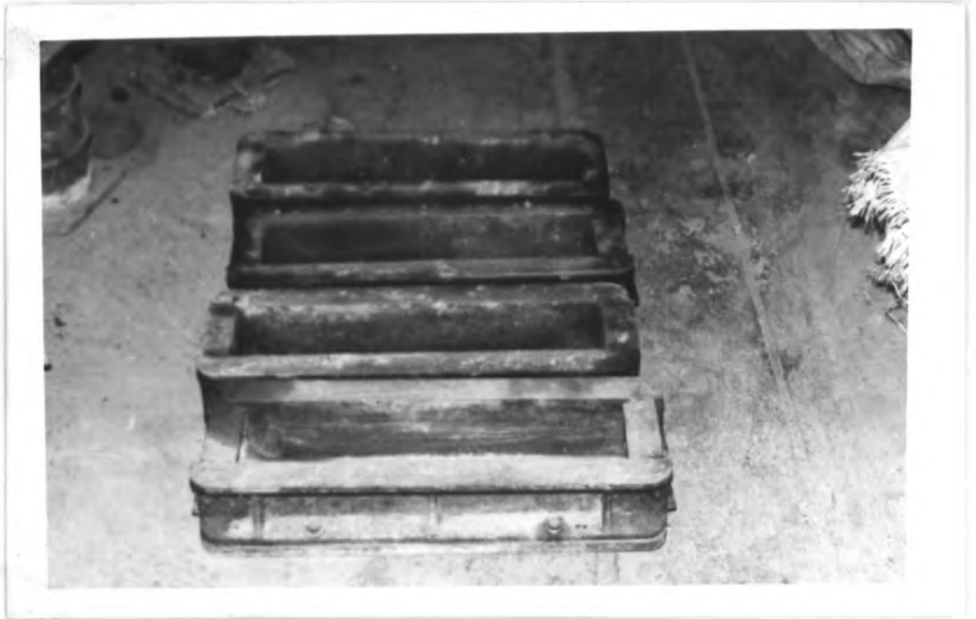
Plate 8.1: Steel moulds used for casting flexure beams.
