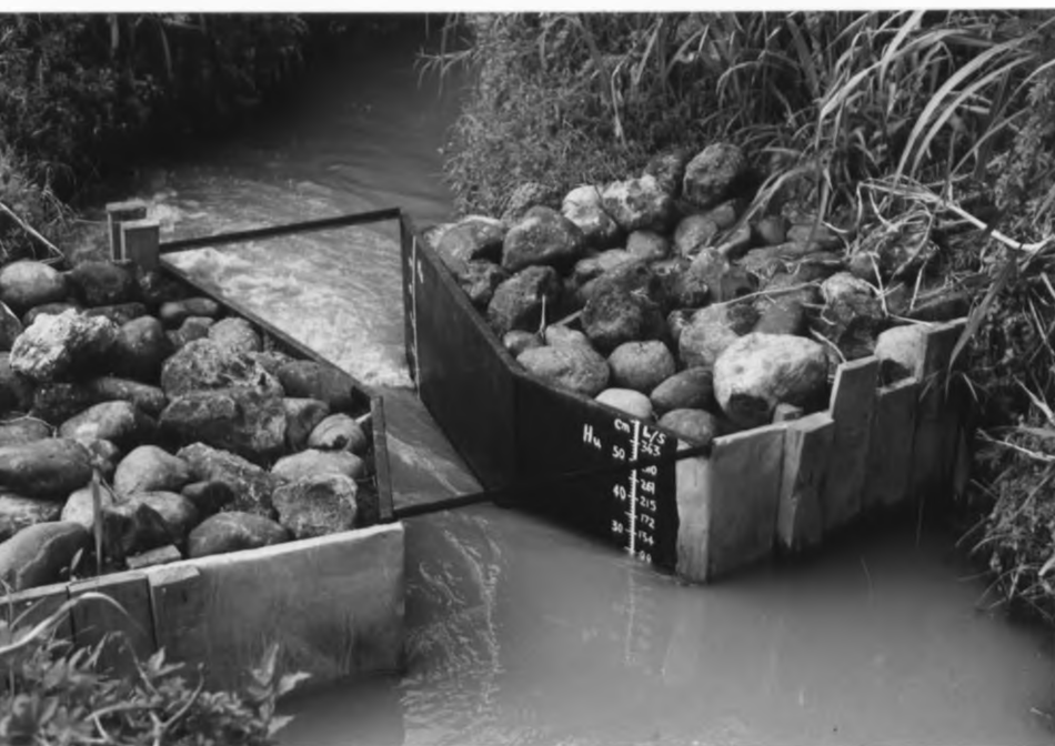
Plate 4.1 40 cm wide cutthroat flume installed in abstraction point No. 25 in operation.
