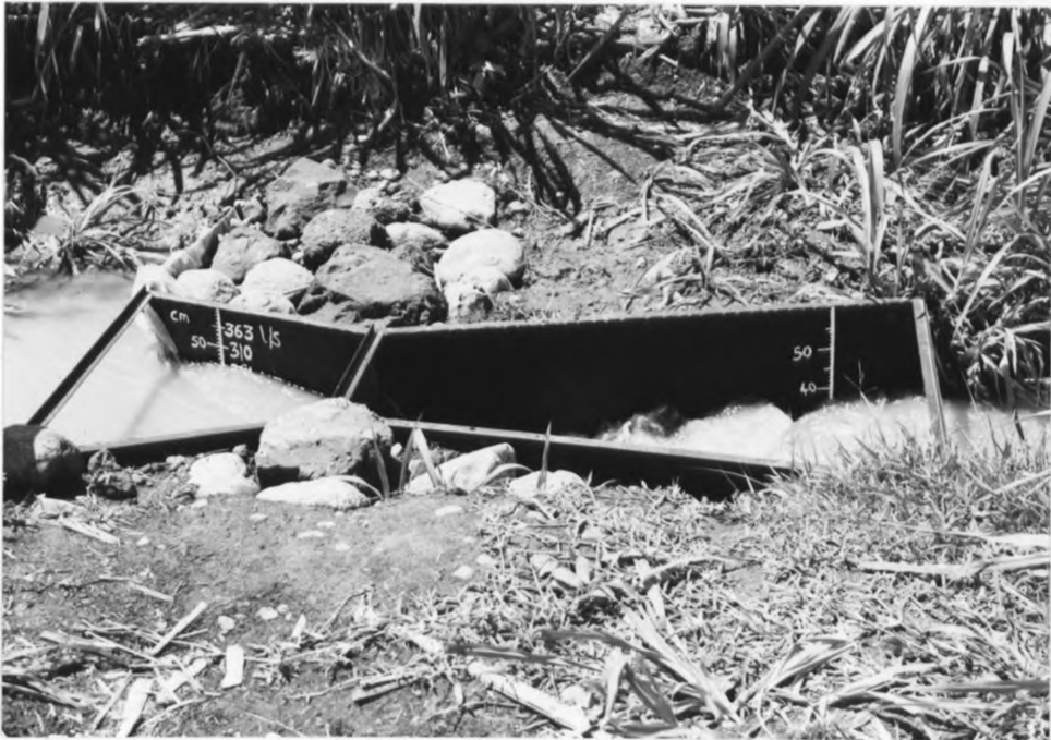
Plate 5.1 Turbulent conditions at the downstream diverging section of a cutthroat flume during high flow.
