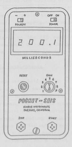
Fig 4.1 POCKET-SEIS ENGINEERING SEISMOGRAPH.
