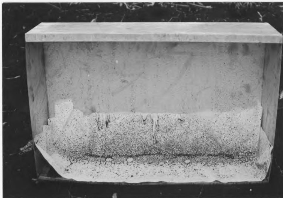
Plate 7. Splash trap showing the trapped soil on the filter paper.
