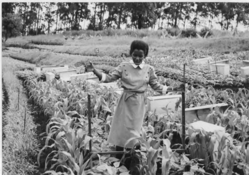
Plate 5. Measuring crop cover using the simple sighting frame.
