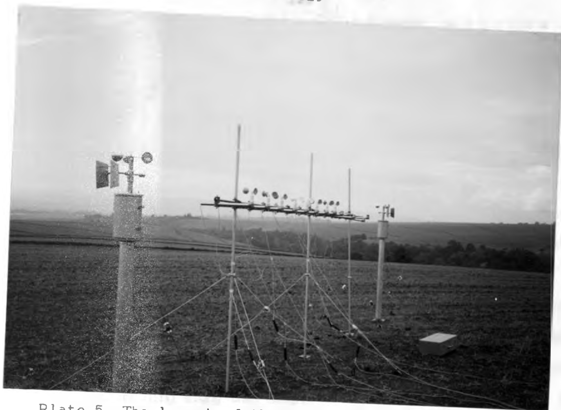
Plate 5. The layout of the wind measuring system during the calibration period (25/1/-3/2/1995) at Embori (Cb3).
