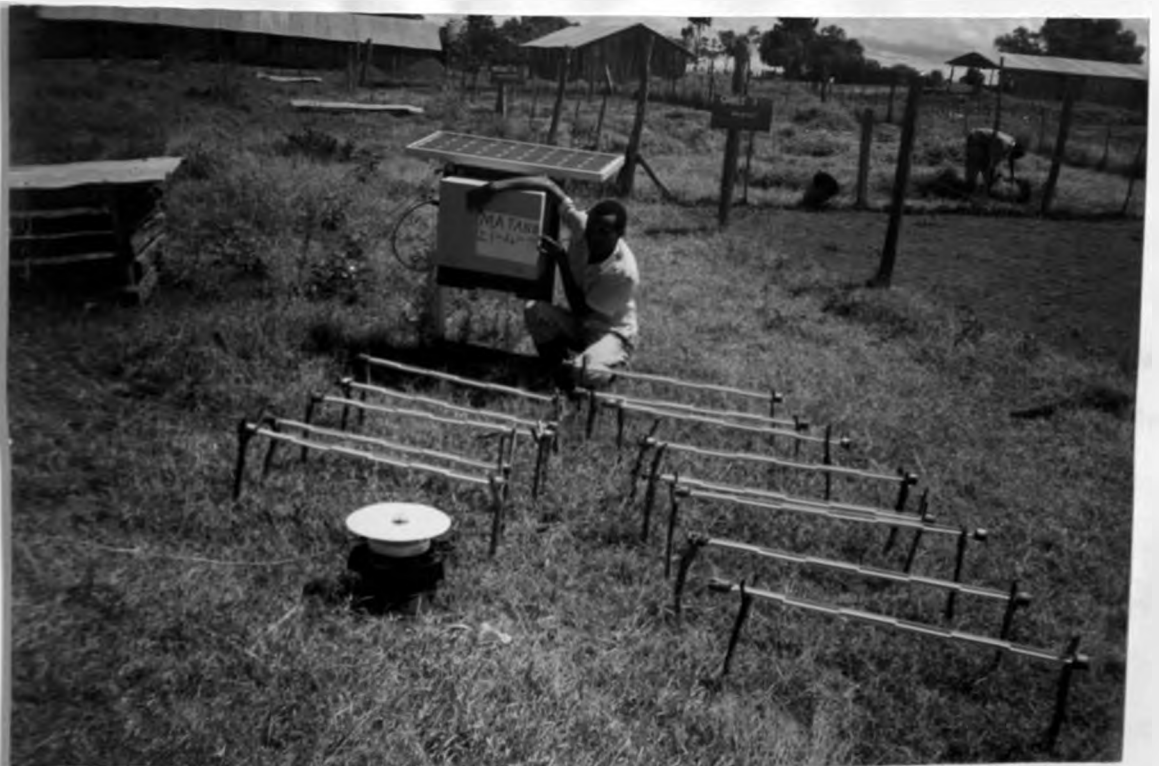
Plate 8. The layout of tube (TSLs) and kippes (kp2) solarimeters during calibration (intercomparisons) in the open next to the solar panel which provided power for the electrical cup anemometers, in October 1991 at Matanya in Cb3 (21/4/1994).
