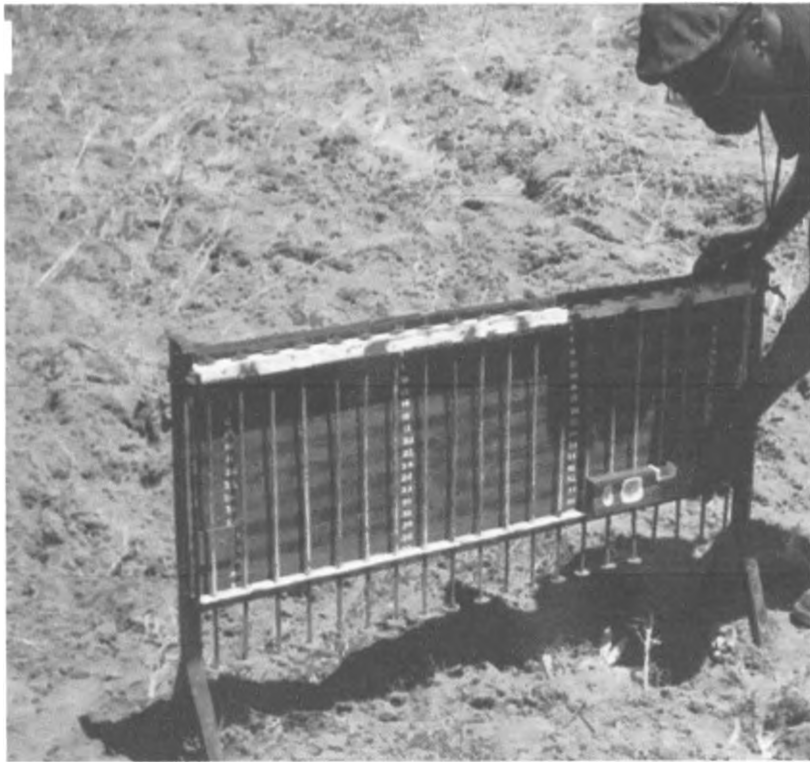
Plate 2.1 Pin-meter instrument being set before measurement are taken.
