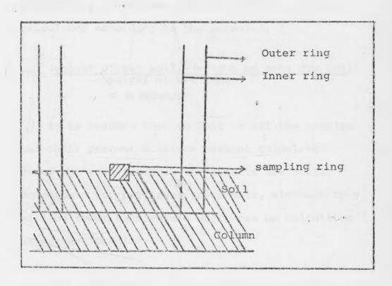
Diag. 3: Placement of the sampling ring in the inner ring.
