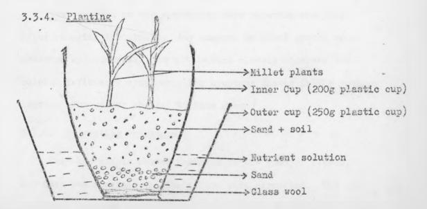
Fig. 1: Apparatus set-up.
